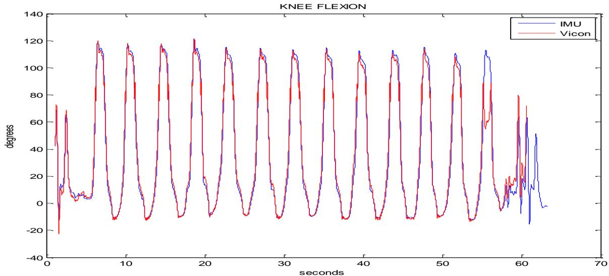
Fig 13: Knee flexion angle after correcting Vicon output for Gimbal lock
