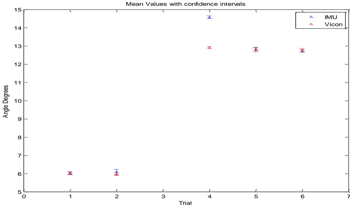
Fig 8: Mean values of pitch across trials: IMUs held static and tilted in alternation
