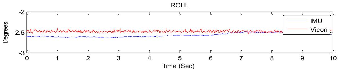
Fig 4: Roll angles when IMU was placed straight and held static at 2.5° (Head)
