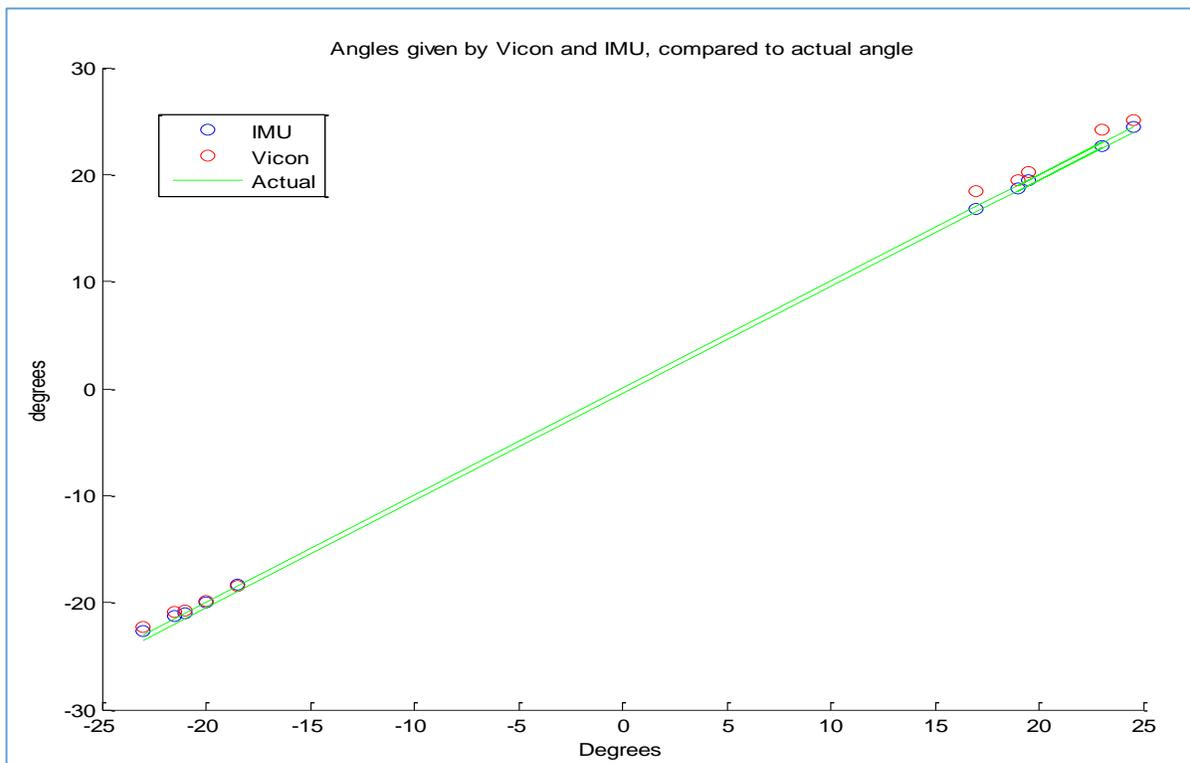
*Fig 2: Peak values of Roll angle from Vicon and IMU across trials. X axis denotes the angles set for different trials. Vicon results for positive angles have a higher degree of error due to occlusion of the Vicon cameras by the Logitech camera that was placed near the markers.*
