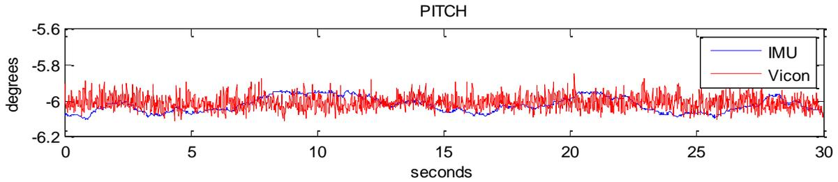
Fig 10: Pitch angle when IMU was placed static and straight in the wooden setup, IMU defined as head.
