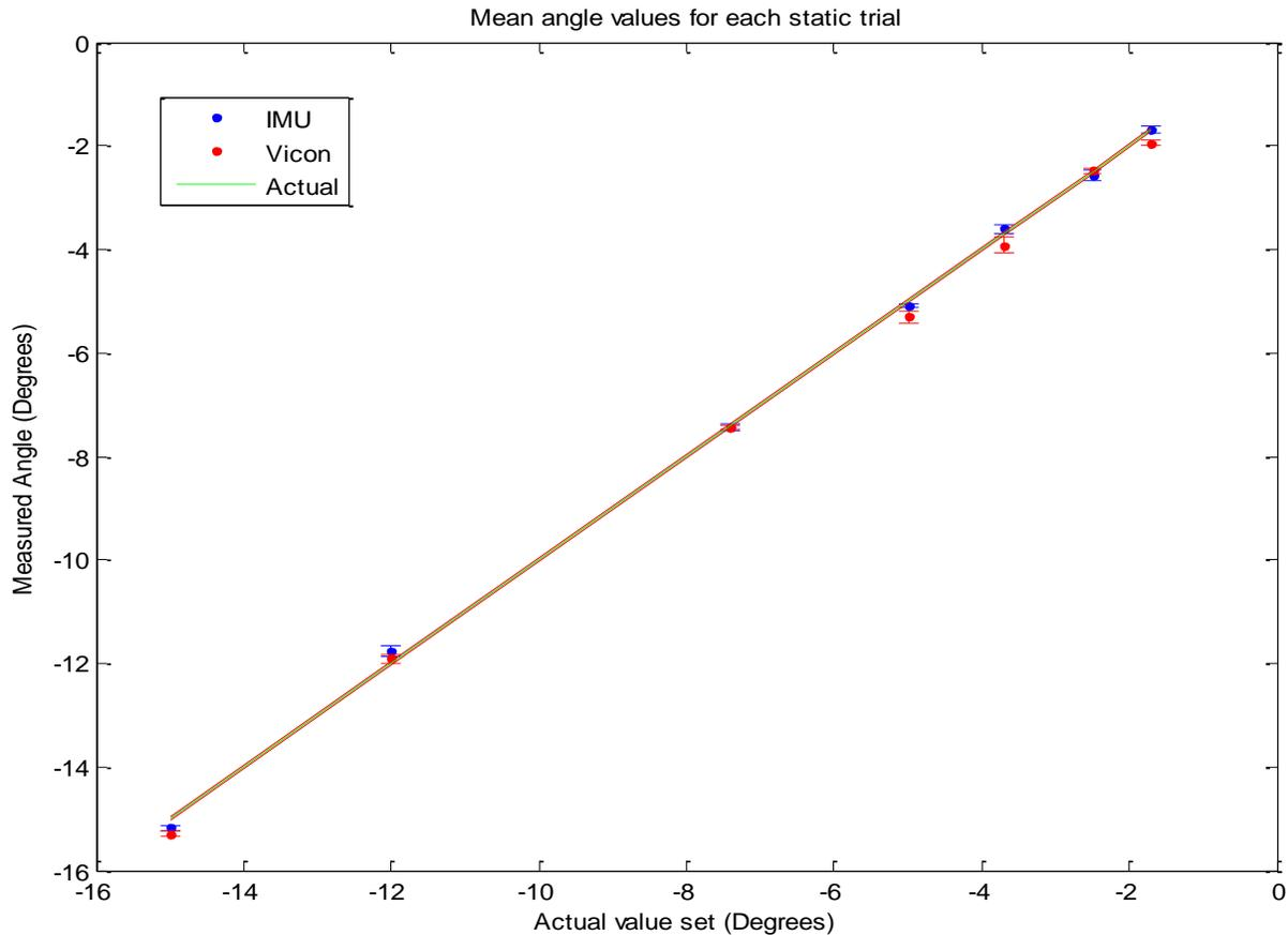
Fig 5: Mean Roll angles across trials when IMU was placed straight and static. Red line denotes the error margin of  $\pm 5$  mm that was considered while calculating the height using laser range finder. X axis denotes the angles set across different trials.
