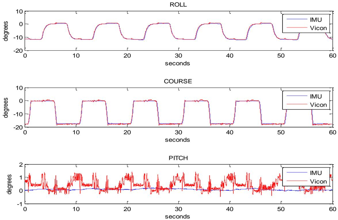
Fig 6: Dynamic Trials: Roll, Pitch and Course angles: Sensor placed upright and defined as head.
