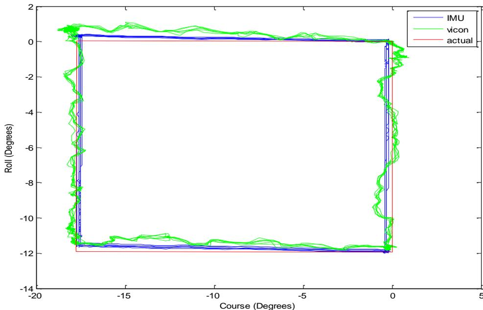
Fig 7: Roll versus Course outputs of MyoMotion and Vicon over a period of 60 seconds
