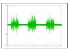
Fig. 33: EMG raw recording contaminated by power hum noise
