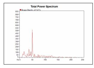
Fig. 32: The total power spectrum of a hum contaminated EMG recording: The high power peak at 50 Hz (European, 60Hz American) identifies the noise contamination of the recording, typically due to increased electrical ground noise of the power net within the selected room (also see fig. 33)
