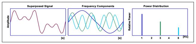
Fig. 56: Model of frequency related signal decomposition based on FFT. The signal on left side contains 3 underlying waves (middle): a sinus wave at 1 Hz, another at 3 Hz and finally one wave at 5 Hz. The power distribution (right) indicates Power of different magnitudes at these frequencies. Adopted & redrawn from 3, p. 24
