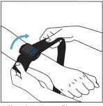
1. Place the MyoMotion™ sensor in the strap cradle. Begin to wrap the strap around the segment.
