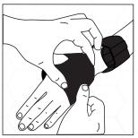
3. Wrap the glove over the sensor and pull tight. Affix the loose end of the glove with the Velcro patch.
