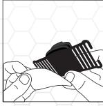
1.Place the MyoMotion™ sensor in the 2. Remove the liner from the tape. Torso adapter. Place doubled sided tape on the backside of the adapter.
