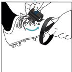
1. Place the MyoMotion™ sensor in the 2. Wrap the band over the MyoMotion™ shoe adapter cradle. Slide the shoe sensor and under the shoe. Be sure to adapter hook under the first lace of the shoe.
