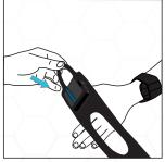
Place the MyoMotion™ sensor in the glove cradle. Place the glove so the thumb goes through the small hole of the glove.
