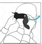
1.Place the MyoMotion™ sensor in the 2. Wrap the free end of the strap completely around the subject's head.
