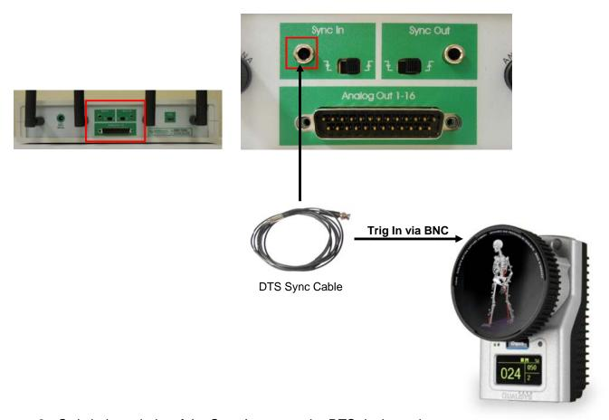
2. Switch the polarity of the Sync In port on the DTS desk receiver to the falling edge (high to low) by moving the switch to the left side
