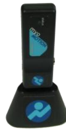
Figure 2: myoMOTION Clinical Receiver (Part# 684)
