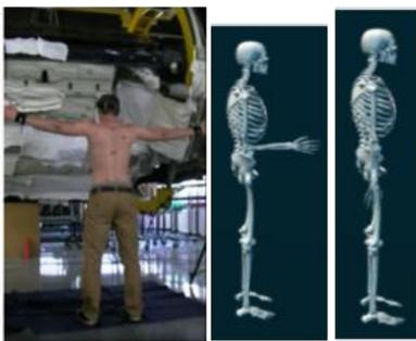
Figure 4: calibration pose; left side: Vicon; middle: MyoMotion: arms flexed; right side: MyoMotion: standing straight
