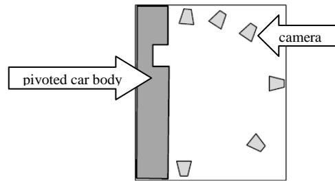
Figure 2: Camera positions for collecting motion data with Vicon
