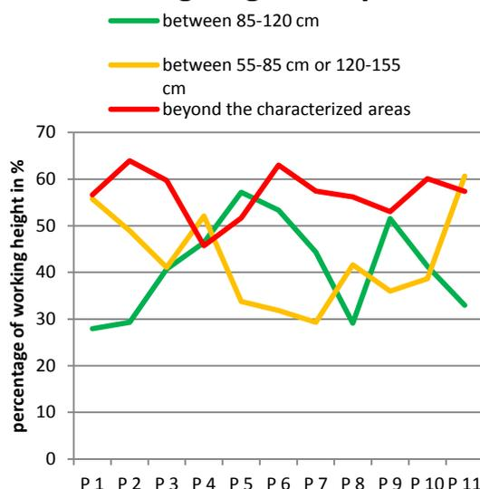
Figure 8: Working height analysis based on motion capture data from the Vicon system
