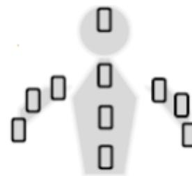
Figure 3: Positions of the ten inertial sensors located at the upper body
