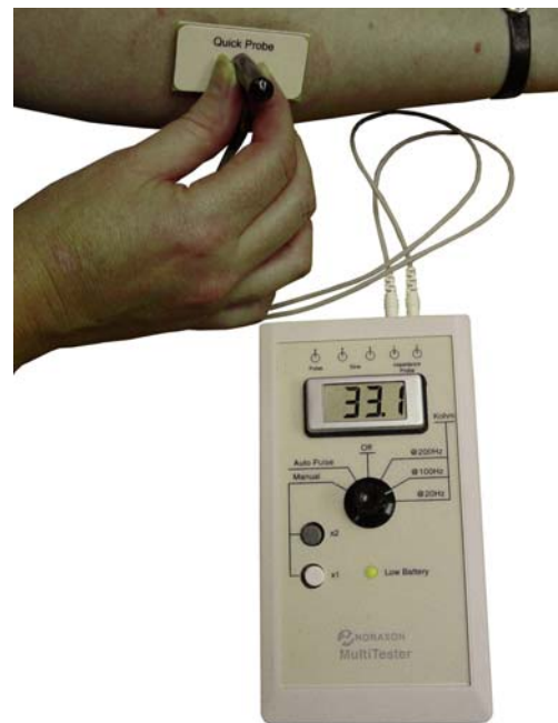
Figure 7: Impedance Measurement Mode using the Quick Probe Lead Set
