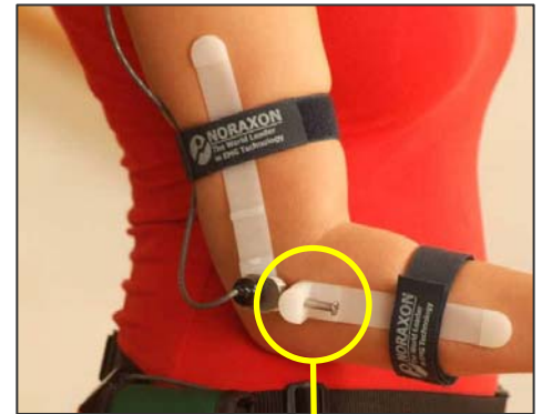
Gliding mechanism to compensate axis motion
