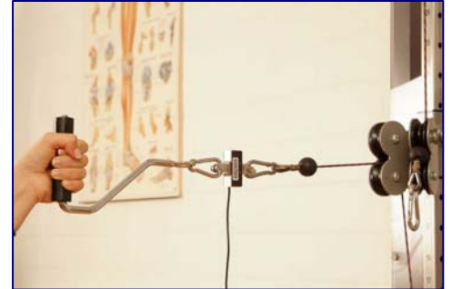
The sensor can be integrated with most cable machines
