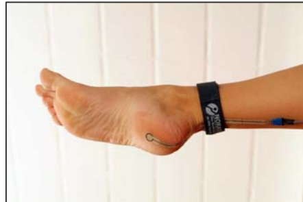
FlexiForce mounted to the heel, suitable for gait studies, impact testing jump and sports performance
