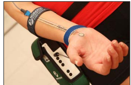
FlexiForce mounted to hand bones, allows detecting of hand and grip pressure force.
