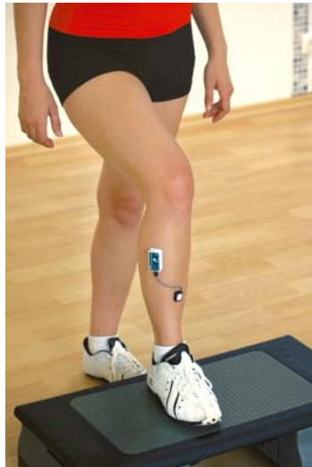
The Accelerometer is mounted (double sided adhesive tape) to the tibia bone, addressing acceleration data in gait analysis
