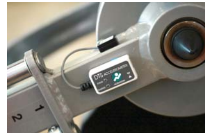
The accelerometer is mounted to a lever arm of a weight stack training machine, addressing vibration effects within axis rotation
