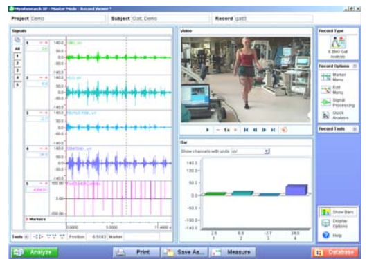
Measurement monitor with raw and real time processed data, combined video and feedback window.
